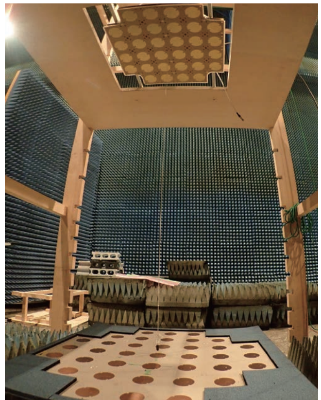
Photo 2: Experimental device for sending and receiving electricity inside an anechoic chamber.
