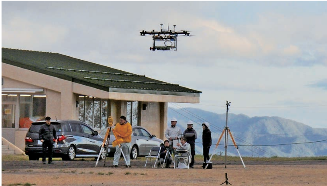
Photo 1: Flight experiment for 16-blade large-scale unmanned aerial vehicle. It is able to fly for 7 minutes with a 10kg load. To extend the flight time, lighter machine parts will be indispensable.
